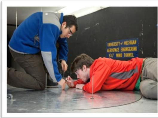
This 5'x7' tunnel is one of the largest in the area, a subsonic low turbulence tunnel capable of operating at over 150 mph. We are interested in measuring the aerodynamic resistance on our vehicle at different speeds that will occur during the race. We ran measurements up to 120 mph, though we don't plan on getting anywhere near that during competition! This high speed comes from the Reynolds number; our scale model is one quarter of the real size, so we have to run tests at four
