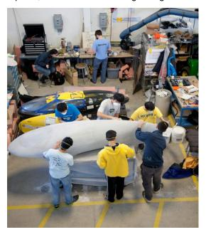
vehicle, we build many pieces of the vehicle individually and once they're complete, assemble the finished single vehicle in its entirety. Instead of permanently fixing every element into the vehicle, each part is attached by a mounting point previously set into the carbon of the body. This allows more time for testing and optimizing specific aspects individually.
