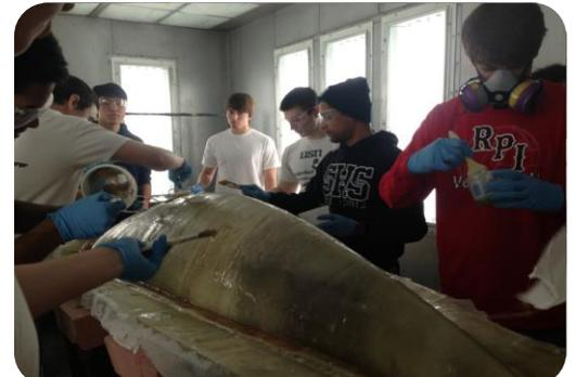
The chopped fiberglass is made up of fiberglass strands held together by an adhesive. It provides stiffness to the female mold, but we use the biaxial weave fiberglass mat for greater strength. It's imperative that we do not put too much resin on at once; the exothermic reaction between the resin and hardener has occasionally made the mixing cups that we use start smoking! We can actually feel the warmth coming off the mold if we lay our hands on it.
