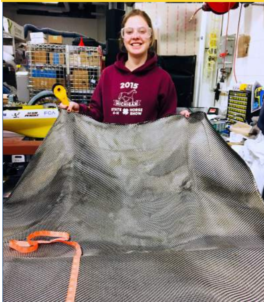
Body Team member Taylor Larsen prepares carbon fiber to make Magnolia's driver canopy, the top piece of the body that sits above the driver's head.
