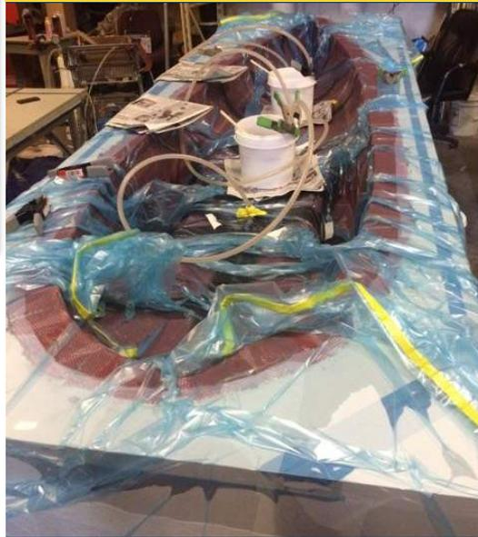
The bottom half of the new battery-electric car Magnolia, made by Michigan Fiberglass, has finished curing and has had aluminum parts laid in it. The body was pulled out of the mold and has been returned to our workspace at the Wilson Student Team Project Center. The team is ready to construct and assemble Magnolia.
